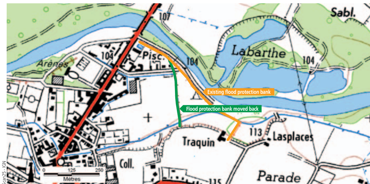
Restoration of the three hectares of flood plain by moving back flood protection banks, representing an additional storage area for 50,000 m 3 of floodwater.
